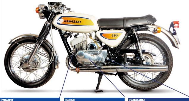
Exhaust header to cylinder joints can give trouble when the steel collars of the header pipes seize onto their studs.
